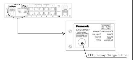
Switch two types of Base mode s and their LEDs in the following way:
