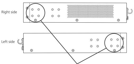
Screw holes for fixing the 19-inch rack mount brackets
