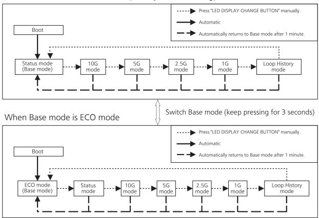
\*The Base mode is maintained even after the power is turned OFF.
