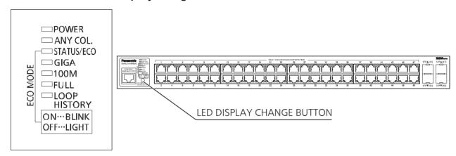
Using "LED DISPLAY CHANGE BUTTON" on the front panel, you can switch the following operations: indication of a connection status with a connected terminal (Status mode), indication of communication speed at 1000 Mbps (GIGA mode), indication of communication speed at 100 Mbps or 10 Mbps (Speed mode), indication of transmission mode of full-duplex or half-duplex (DUPLEX mode), indication of a port having a history of loop occurrence (Loop History mode), or turning off LEDs of all ports (ECO mode).
