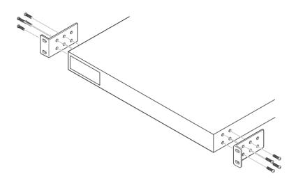
The main unit can be placed 20 mm back on the rack by changing the bracket fixing position.
