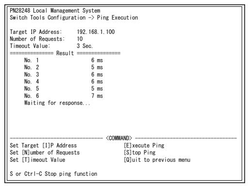
Fig. 4-86 Display during Ping Execution
