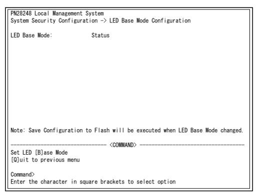
Fig. 4-22 LED Base Mode Configuration
