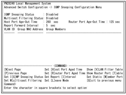
Fig. 4-56 IGMP Snooping Configuration
