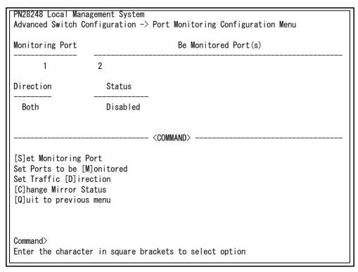
Fig. 4-42 Port Monitoring Configuration
