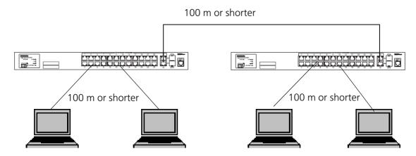
Figure 3-1 Connection configuration example
