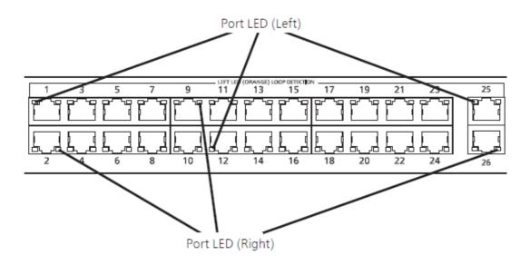
Figure 1-1 Port LEDs
