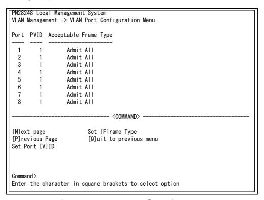
Fig. 4-38 VLAN Port Configuration Menu
