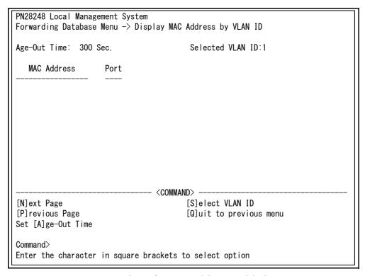
Fig. 4-28 Display of MAC Address Table by VLAN
