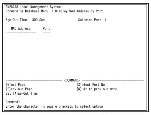
Fig. 4-26 Display of MAC Address Table by Port
