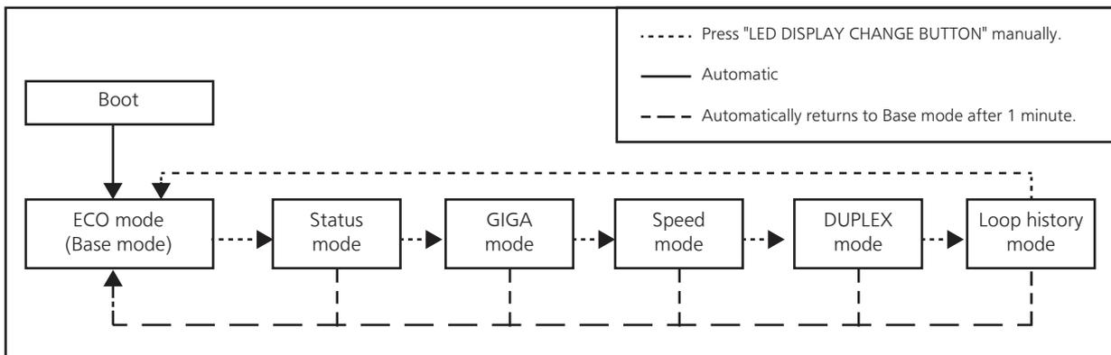
※The Base mode is maintained even after the power is turned OFF.
