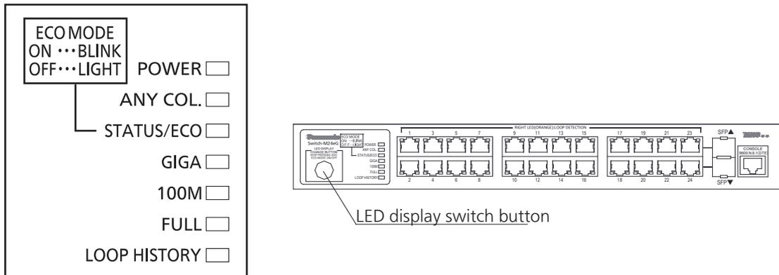
You can display the following items using the LED display switch button.
