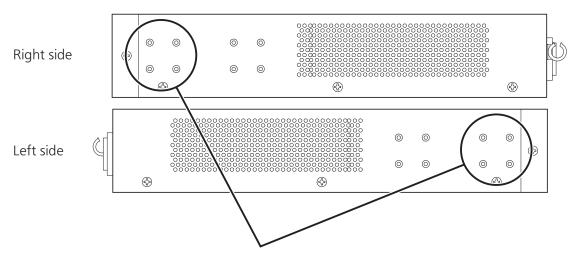
Screw holes for fixing the 19-inch rack mount brackets
