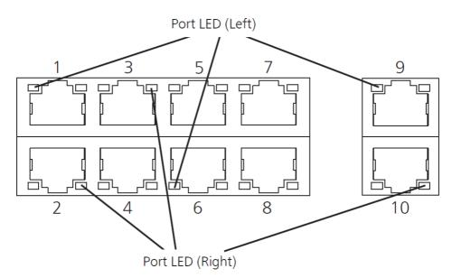
Figure 1-1 Port LEDs
