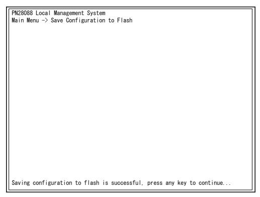
Fig. 4-91 Save Configuration to Flash Screen: Completed
