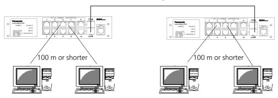
Figure 3-2 Optical fiber cable connection example
