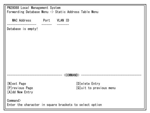
Fig. 4-24 Addition or Deletion of MAC Address
