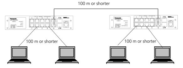
Figure 3-1 Connection configuration example
