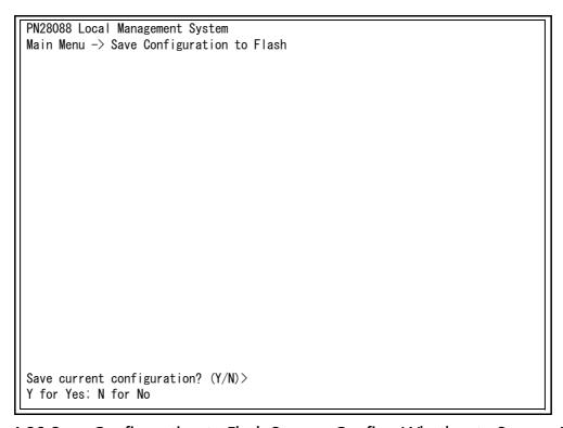
Fig. 4-90 Save Configuration to Flash Screen: Confirm Whether to Save or Not
