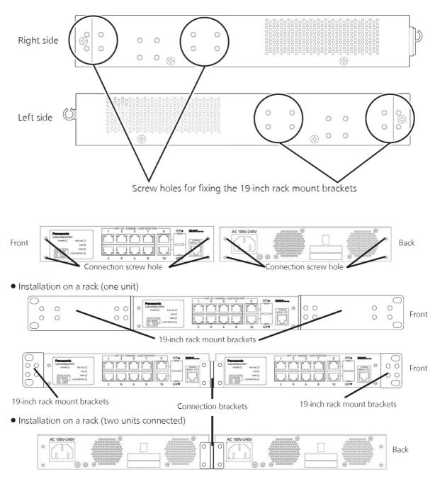
Figure 2-1 Installing in rack
