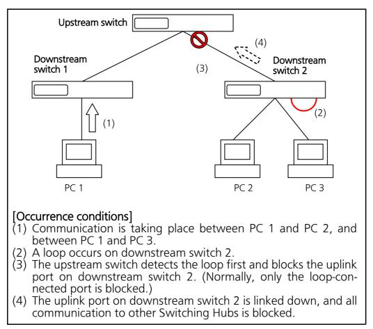
Figure 5-2 Notes when using the Loop detection and blocking function
