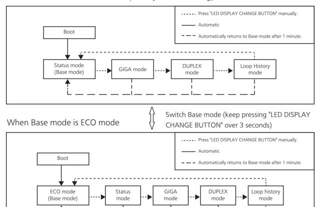
\*The Base mode is maintained even after the power is turned OFF.
