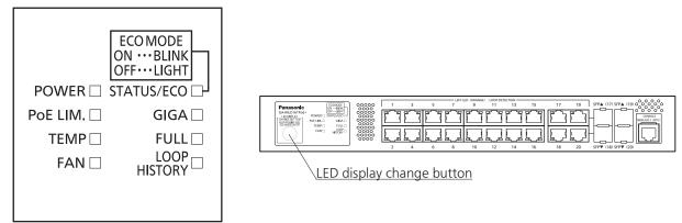
You can display the following items using the LED display switch button. Display for the connection with a connected terminal (Status mode), Display for the 1000 Mbps transmission rate (GIGA mode), Display for the full-duplex or half-duplex transmission system (DUPLEX mode), Display for ports with a loop history (Loop history mode), All port LED lamps can be turned OFF (ECO mode).
