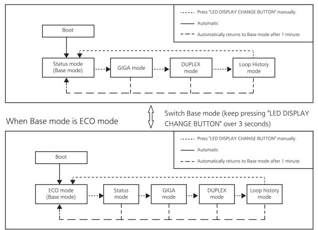
\*The Base mode is maintained even after the power is turned OFF.
